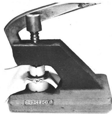
SEIKO tightening tool (S-160)
